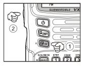
3. When you are satisfied with the Squelch threshold setting, press the **PTT** key momentarily to save the new setting and exit to normal operation.
