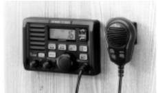
Output power : 25 W or 1 W (at 13.8 V DC) • Modulation system : Variable reactance freq. mod.
